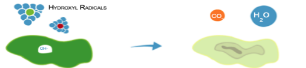
THE HYDROXYL RADICALS WORK TO RUPTURE THE SURFACE MEMBRANE LEADING TO MALFUNCTION AND EVENTUAL DEATH OF THE PATHOGEN CELL WITH ONLY CARBON DIOXIDE AND WATER VAPOR REMAINING.
